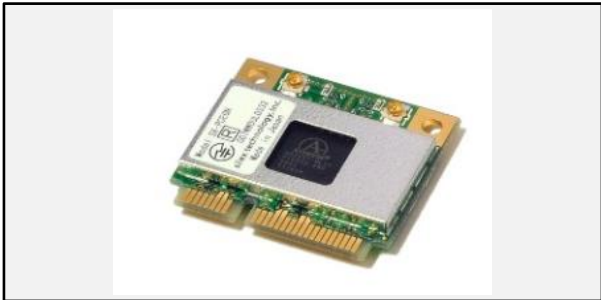
Figure 1. With Silex Technology's 802.11b/g/n Mini-PCI Express Radio Module embedded in Lowrance's marine multifunction display, boaters are no longer tethered to the display's location on the boat .
